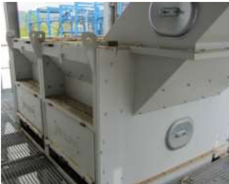
Image 5: The disc screen removes wood pieces that are too long. The sorted excess lengths go straight to a container.
