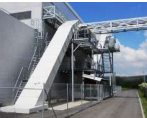
Image 3: Vecoplan supplied a tailor-made storage, dosing and transport solution. Scraper chain conveyors are an important element of the solution.
